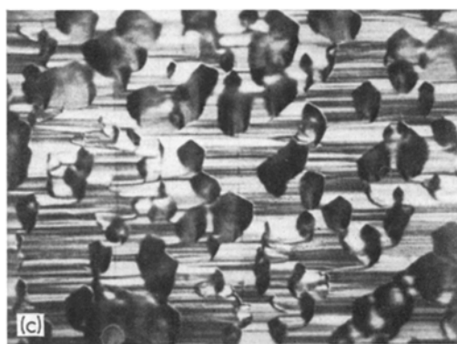
Figure 3 Optical surface micrographs of thin layers grown at (a) 500°C, (b) 650°C and (c) 800°C using an H_2 flow of 0.75 l min^{-1} and a source temperature of 1120°C.
